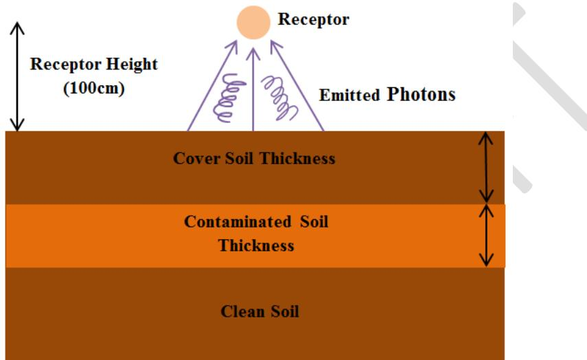
**Figure 1: Geometry of Gamma Shielding Factor Calculation**
